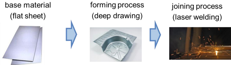
Fig. 1. Typical processing chain showing the consecutive forming and joining processes.
