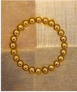
Fig. 3. Surface polished and sanded and etched with acid and oxidized, pulsed green laser
