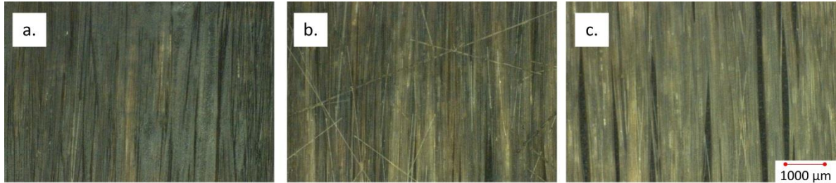
Fig. 4: Behaviour of selective matrix removal at a. Parameter set 1 with 6.99 J/cm 2 and 50 % overlap, b. 12.24 J/cm 2 and 50 % overlap and c. 1.41 J/cm 2 at 93 % overlap. In a. some of the fibres are still embedded in the polymer matrix. In b only a small polymer film left around the fibres and fibre damaging can be observed. In c the fibres are completely freed from polymer
