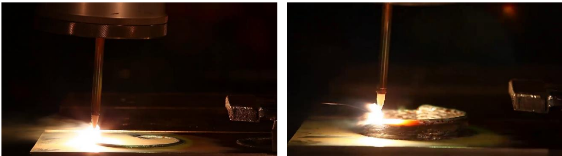
Fig. 5: Wire-based coaxial laser cladding of a circle after one layer (left) and twelve layers (right)
