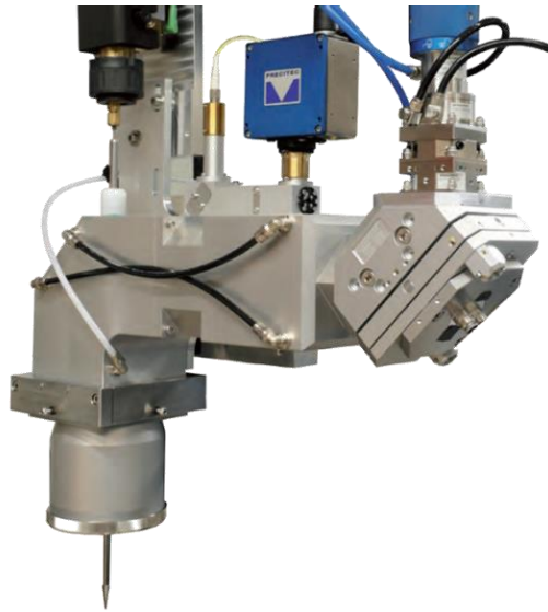
Fig. 1: CoaxBrazer design with attached sensor technology
