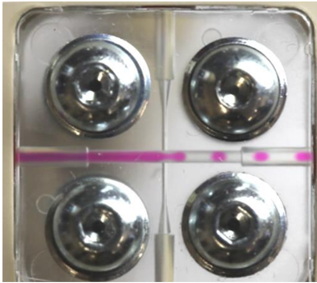
Figure 7: Demonstrator device. The fluid is continuously injected from the left (pink). From the top and bottom channels a separation liquid is injected into the main stream.
