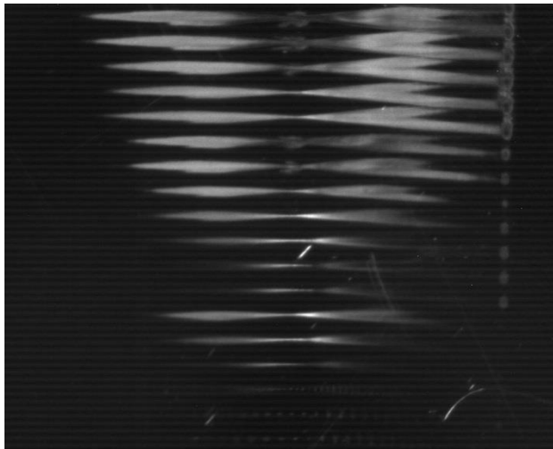
Fig. 2. Traces generated by the D-Scan technique in steel VI 138, with 25 fs laser pulses.
