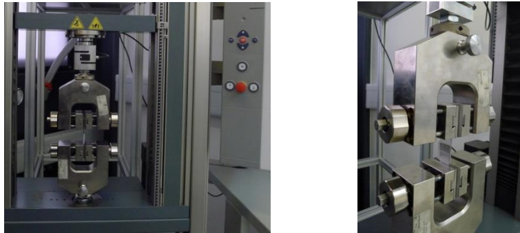
Figure 6. Shear stress tests of polymer metal hybrids.
