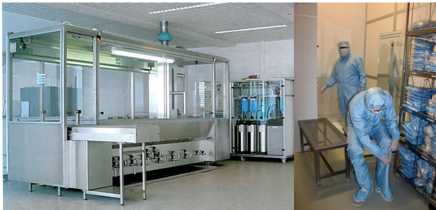
Fig. 1. a) Ultrasound cleaning, b) Preparations to enter the ISO 5 cleanroom
