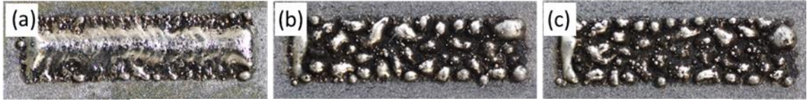
Fig. 4 Optical images of cladding layer surface (a) 30, (b) 40 and (c) 55 \mu\text{m} .
