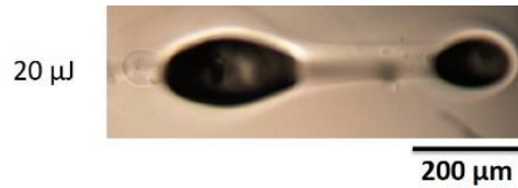
Fig. 2. Microscope top view of cracks in a single line modification obtained with 18-ps laser pulses at 20 \mu\text{J} of pulser energy. The repetition rate is 500 kHz, the translation speed 0.1mm/s.
