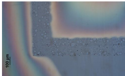
Fig. 7. Microscope detail of an ultrashort laser welded sample along a square path.
