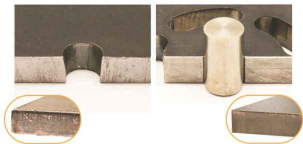
Fig. 2. Comparison of cut results in 10 mm mild steel, hole diameter = 12 mm: left conventional plasma cutting, right plasma cutting with increased constriction (HiFocus Contour Cut)
