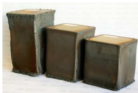
Fig. 8. Cutting samples stainless steel; left: 150 mm, centre: 100 mm, right: 80 mm
