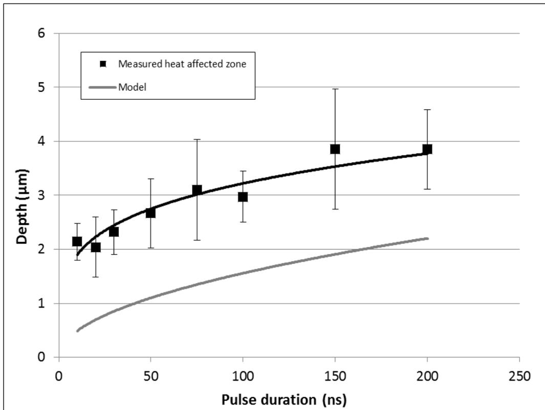
Fig. 4. Heat affected zone characterized in the SEM versus values calculated with the model.
