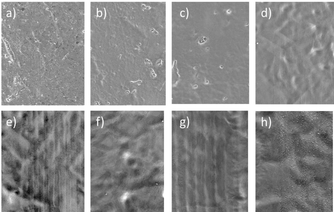
Fig. 1. SEM micrographs from samples (a) not processed ; (b) processed at 20 ns; (c) processed at 30 ns; (d) processed at 50 ns.; (e) processed at 75 ns; (f) processed at 100 ns; (g) processed at 150 ns.; (h) processed at 200 ns.
