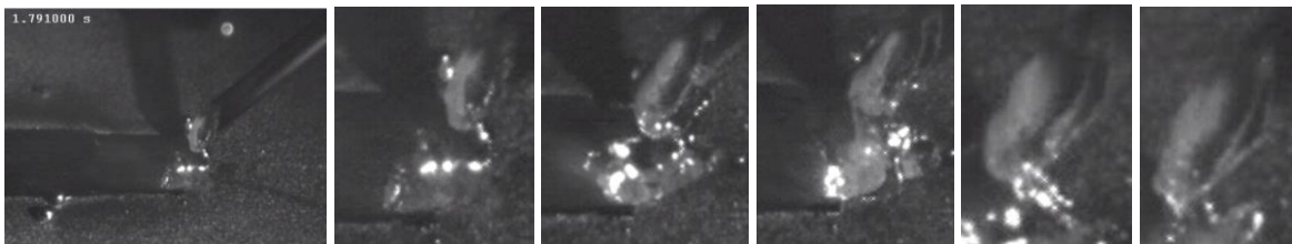
Fig. 3. Survey picture and sequence (time steps: 250 μs) of high speed images of the concave boiling front at the wire tip for a non-oscillating laser beam.
