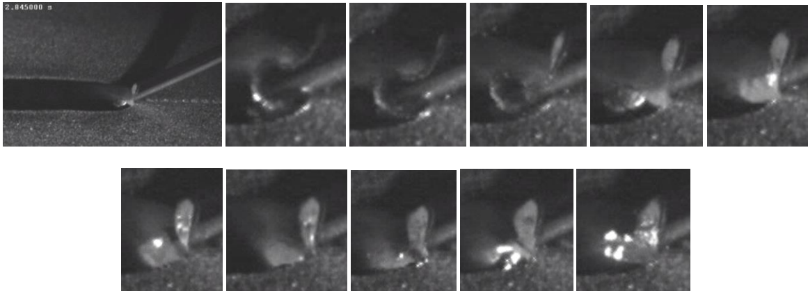
Fig. 5. Survey picture and sequence of high speed images (250 \mu s) when chopping the wire into solid pieces by a laterally oscillating laser beam (60 Hz).
