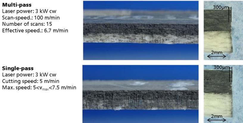
Fig. 7: Cut edges and cross sections of multi-pass and single-pass cuts in welded material of 4.4 mm thickness (GF/PA with 60 weight-% fibre content).
