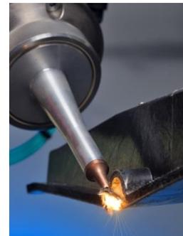
Fig. 9: (a) Cutting speed for trimming the seating structure at the welded edge of the component; (b) Cutting process with a slender nozzle for good accessibility.
