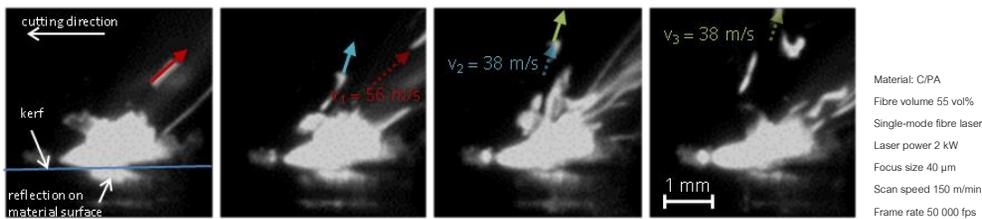
Fig. 5: High speed video of an ablation process, showing particles ejected out of the kerf.
