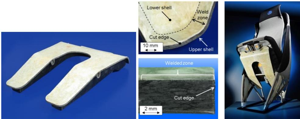
Fig. 10: left: Seating structure and details of the edges; right: Assembled seat with the demonstrator part
