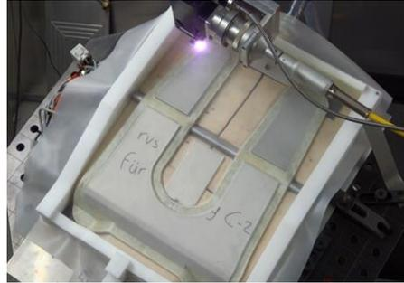
Fig. 8: Structure of the seat components (left) and welding of the components on a articulated arm robot (right).
