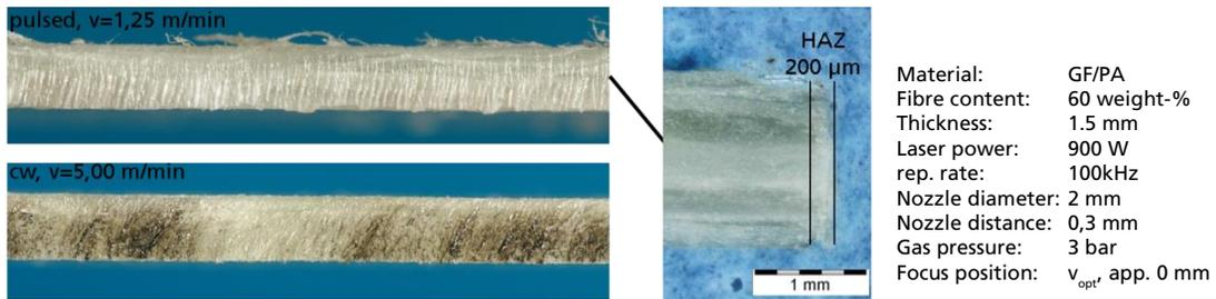
Fig. 6: Cut edge GFRP, pulsed (top) and cw (bottom) processing.
