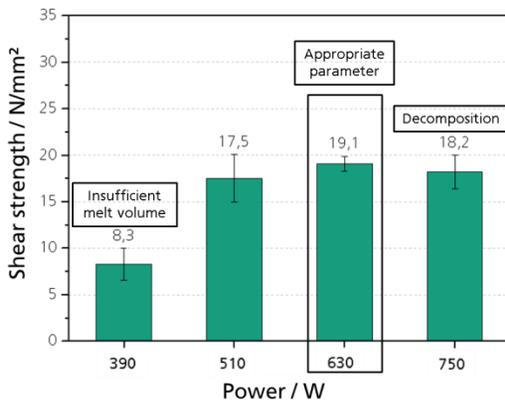
Fig. 2: Welding strength depending on laser power (feed rate 50 mm/s, material Tepex® flowcore 2mm / ~ 60 wt. % glas fibres)
