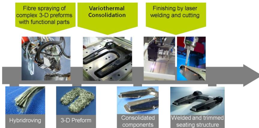
Fig. 1: InProLight process chain for 3-D thermoplastic glass fibre reinforced parts.
