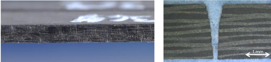
Fig. 3: Cut edge and cross section of a cut sample C/PA, 2 mm thickness, with a ns-CO<sub>2</sub>-laser (average power 1 kW, peak power 60 kW, scan speed 240 m/min, effective speed 0.5 m/min).
