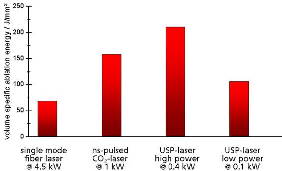
Fig. 4: Volume specific energy consumption for ablating carbon fibre composites, scaled to a fibre content of 60 vol-%.
