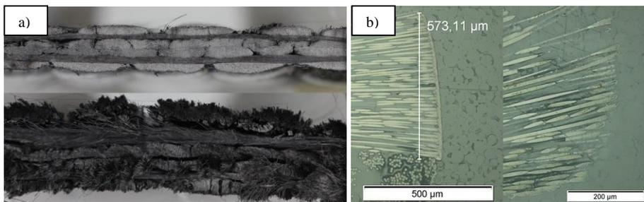
Fig. 4. (a) Cutting area of laser cut non-crimped fabrics, laser power 1kW (top) / 6kW (bottom); (b) Fiber swelling of a 0°-layer (non-crimped fabric), laser power 0,5kW (left) / 5kW (right)
