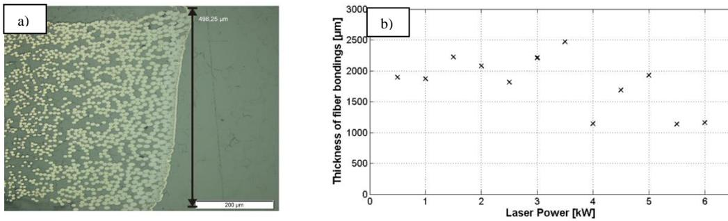
Fig. 3. (a) Fiber bonding; (b) Thickness of fiber bondings at different laser power
