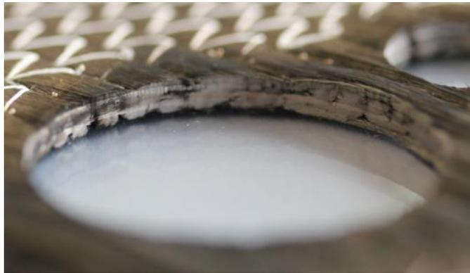
Fig. 5. Cutting edge of laser cutted preform
