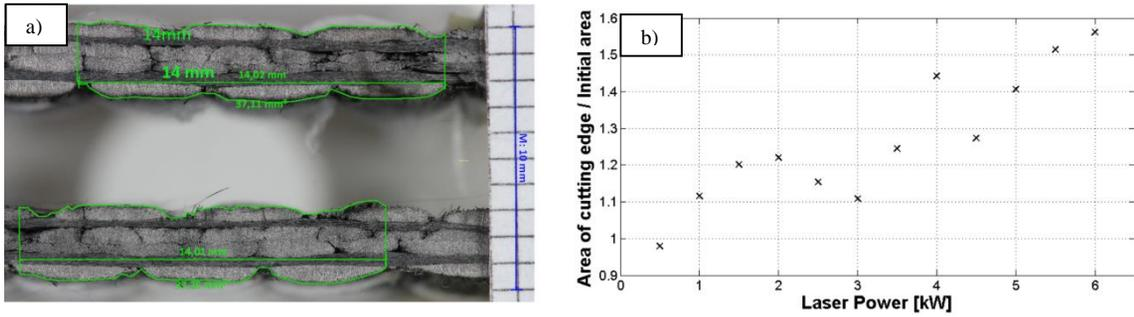
Fig. 2. (a) Measured area of the cutting edge; (b) Area of cutting edge / Initial area at different laser power
