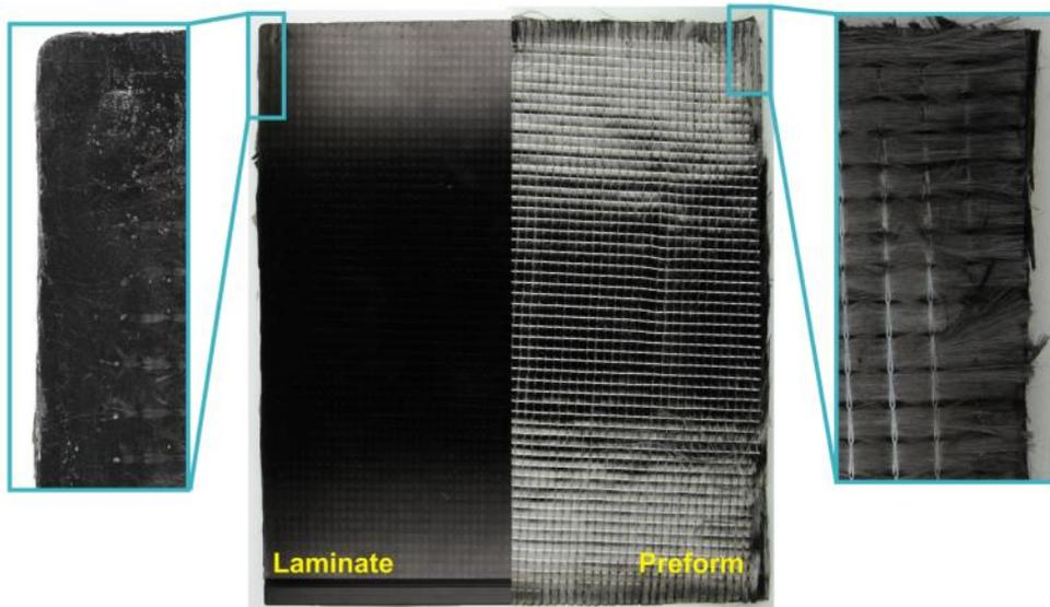
Fig. 6. Comparison of a laser cutted preform (right) and the resulting laminate after RTM infusion (left)
