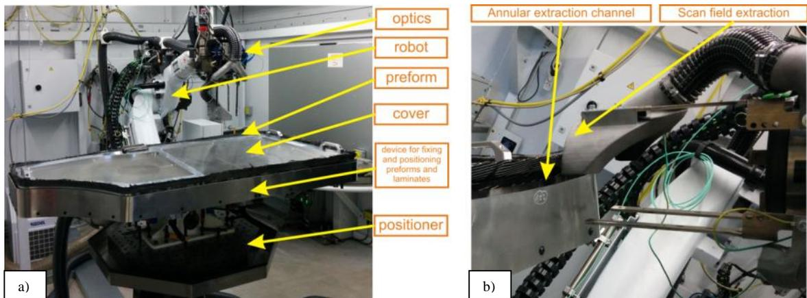
Fig. 7. (a) Experimental setup; (b) concept of emission extraction
