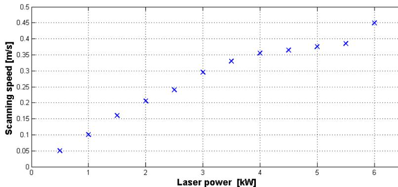
Fig. 1. Necessary scanning speed at increasing laser power
