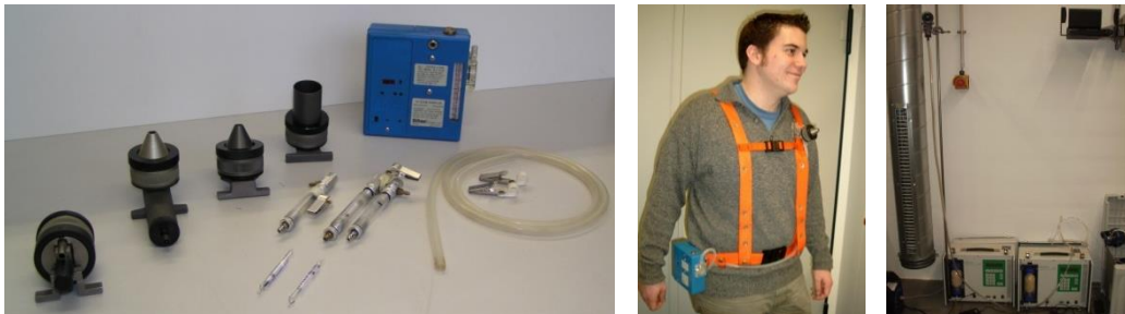
Fig. 9. (a) Occupational exposure assessment sampling strategies and sampling heads, (b) personal, (c) stationary measurement.
