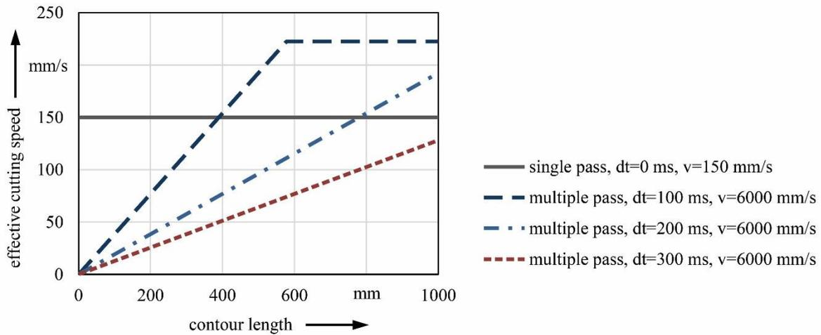
Figure 7: Effective cutting speed as a function of the contour length for the single pass and the multiple pass strategy
