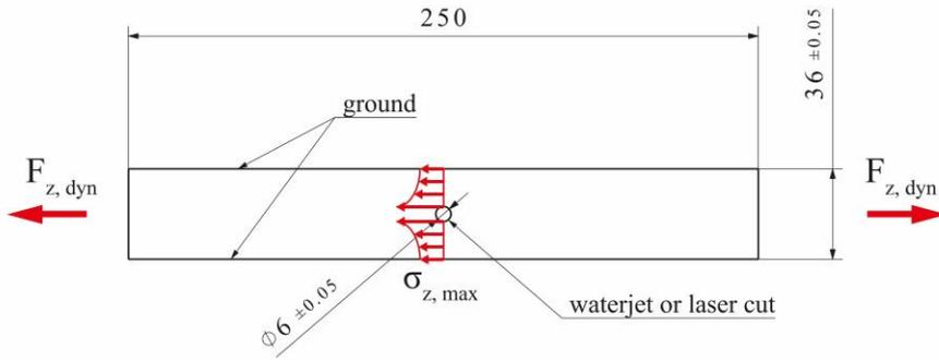
Figure 1: Specimen geometry based on ASTM D5766/D5766M-11; the dynamic load  $F_{z,dyn}$  is applied in the longitudinal direction; the arrows at the critical plane indicate the qualitative distribution of the maximum stress  $\sigma_{z,max}$
