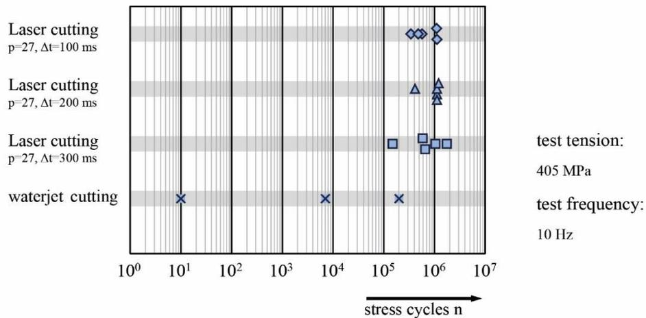
Figure 3: Open hole tensile tests at a dynamic load  $F_{z,dyn}=405$  MPa
