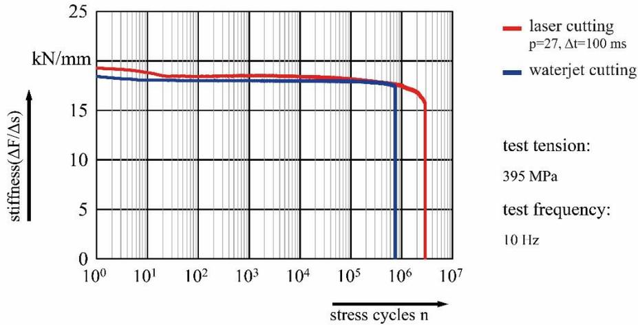
Figure 5: Typical stiffness trend for waterjet and laser cut specimens
