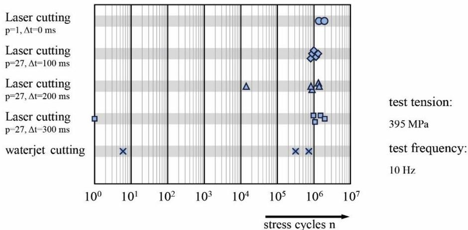
Figure 4: Open hole tensile tests at a dynamic load  $F_{z,dyn}=395$  MPa
