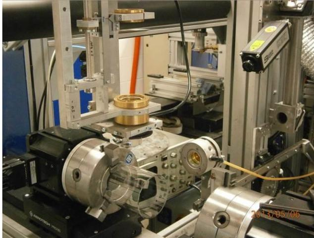
Figure 1: Experimental setup with axis system, optics and pyrometer
