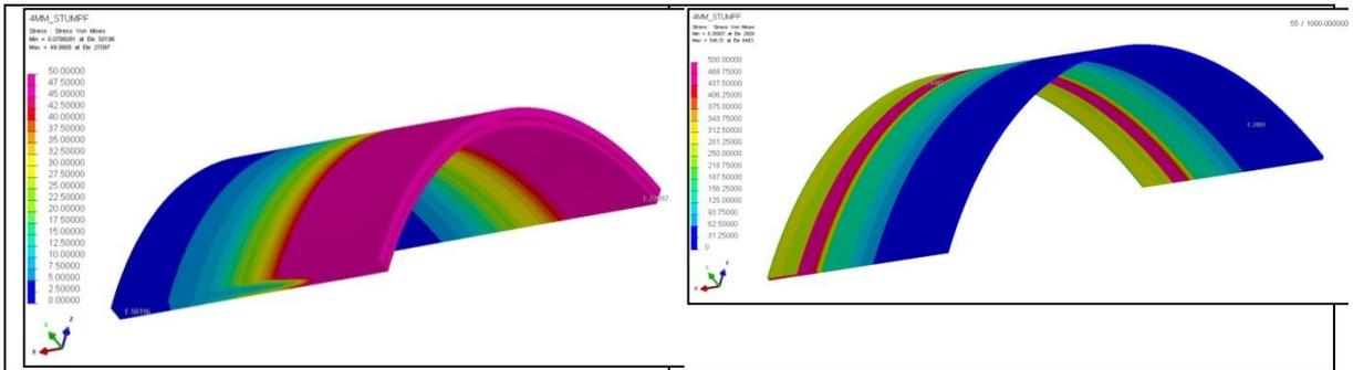
Figure 11: Internal stress [N/mm<sup>2</sup>] in glass (links) and metal
