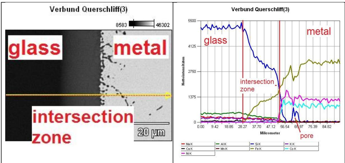
Figure 10: REM-picture and EDX-analysis of the joining zone
