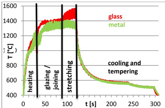
Figure 6: Temperature graph of the joining process
