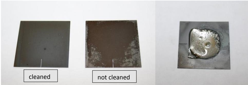
Figure 5: Influence of cleaning to oxidation and glazing
