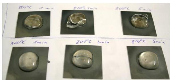
Figure 4: Glazing with a mix of oxides (upper row) and with FeO only (lower row)
