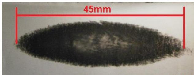
Figure 2: Laser beam geometry (tube  $\varnothing 75 \times 3.2$ )
