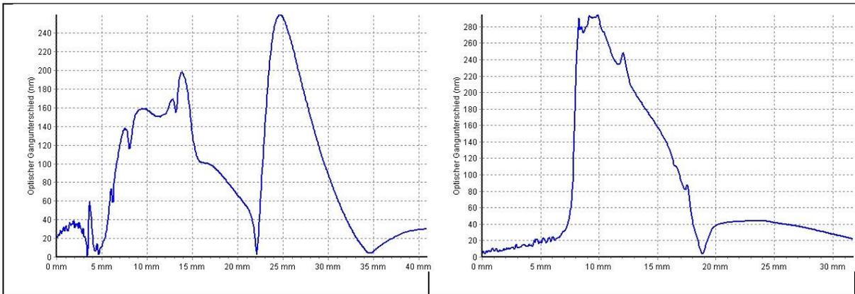
Figure 9: Measurement of stress before (left) and after tempering (right), miscolored map and line scan
