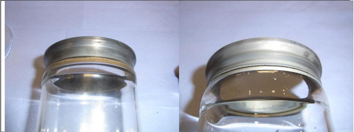
Figure 8: Unadapted bond with a mix of oxides (left) and with FeO (right)
