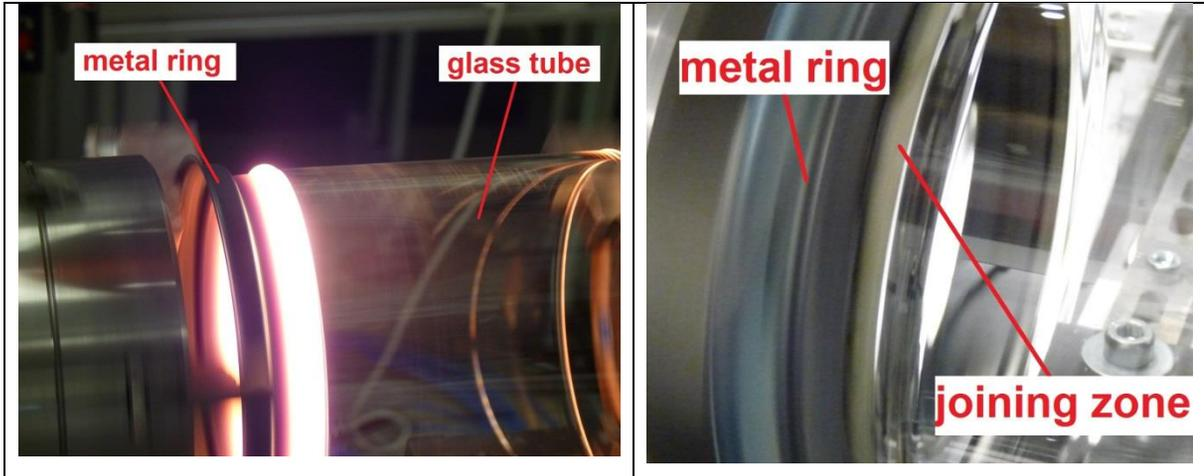
Figure 7: Glazing process and joining zone
