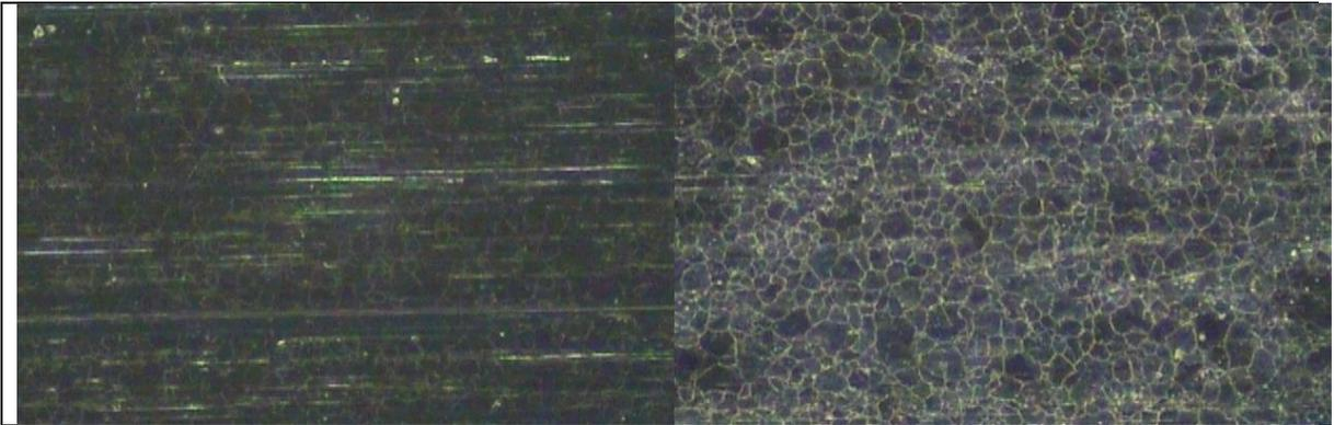
Figure 3: Left not cleaned and right cleaned Kovar surface
