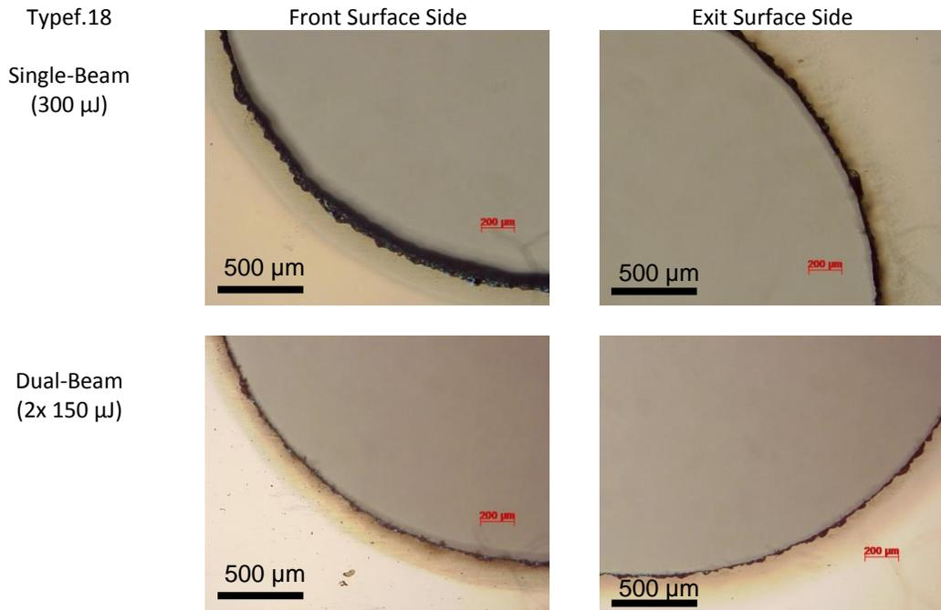
**Fig. 2:** Microscope images of a 0.2 mm thick quartz sample after internal contour cutting (ca. 2 mm diameter) using a nanosecond DPSSL system at 532 nm and a LMTB trepanning system type1.f18 in a single-beam (top) and dual-beam (bottom) configuration.
