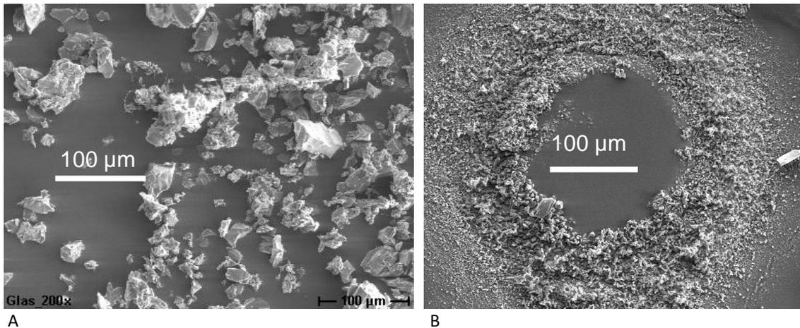
**Fig. 6:** SEM images of the glass dust or particles collected during rear side laser machining of soda-lime glass at 532 nm at different pulse width. **A:** 25 ns, **B:** 7 ps.
