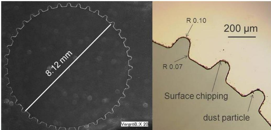
**Fig. 3:** Microscope images of a 0.17 mm thick quartz sample after a complex internal contour cutting (ca. 8 mm diameter) using a sub-ns DPSSL system at 532 nm and a LMTB trepanning system type1.f18 in a single-beam configuration.
