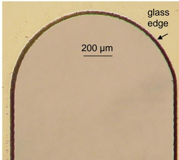
**Fig. 5:** Microscope images of a thin-sheet soda-lime glass sample after laser machining for internal contour cutting. A 0.1 mm thick soda-lime glass was machined using ultra-short laser pulses at a wavelength of 1025 nm, pulse width = 0.4 ps, energy = 50  $\mu\text{J}$  per pulse at 30 kHz.
