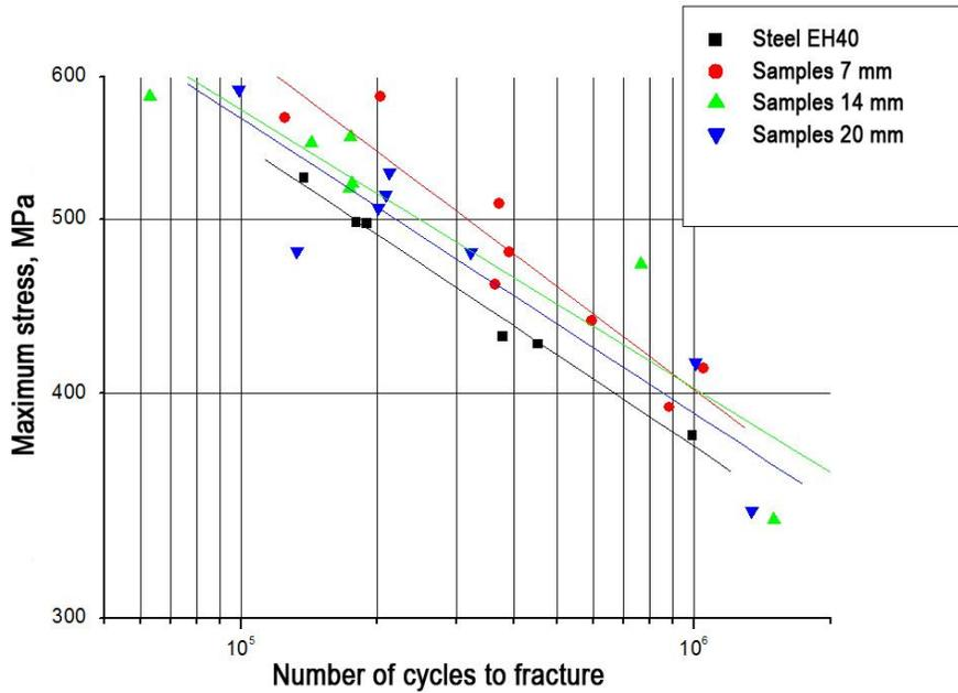
Fig. 2. Results of welding sample fatigue testing
