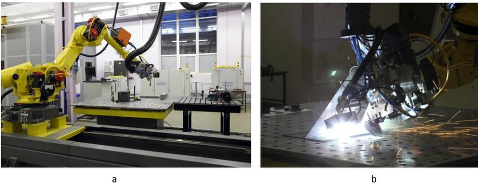
Fig. 5. Robotized complex for laser welding and cutting in various spatial positions: (a) general view of the complex, (b) hybrid laser-arc welding process
