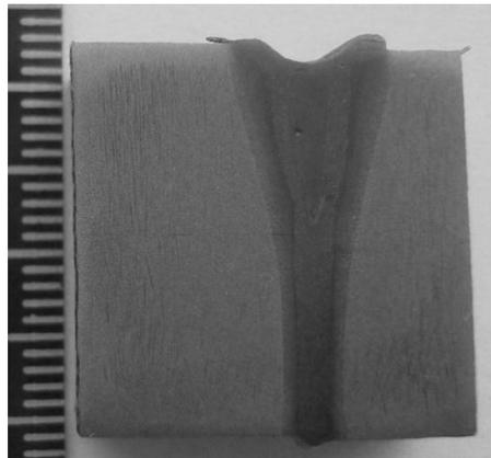
Fig. 6. Macrostructure of the vertical welding seam
