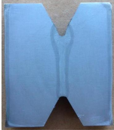
Fig. 7. Macrosection of high strength shipbuilding steel, 48 mm thick
