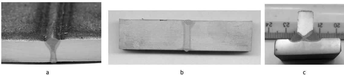
Fig. 3. Macrosections of hybrid laser-arc welding joints: (a) butt-joint 7 mm and (b) 20 mm thickness, (c) T-joint 7 mm/7 mm thickness
