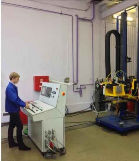
Fig. 8. Technological complex for automatic vertical hybrid laser-arc welding
