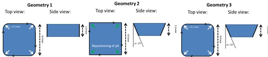
Figure 6: Geometry 1: Cutting geometry used for 2-axis cutting. Geometry 2: Cutting geometry used for cutting with a 2-axis system with clearance angle. Geometry 3: Cutting with 5 axes.
