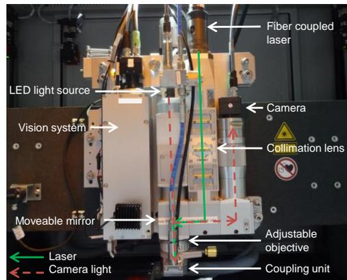
Figure 1: Setup of the optical head which couples the laser into the water jet.
