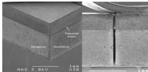
Figure 14: Left: SEM picture of a wire cut and wet laser cut (Laser MircoJet® cutting) PCD showing excessive EDM erosion at the PCD/HM interface. Right: An SEM picture of a cross-section through a parallel sided 50 μm wide kerf in 1.6mm PCD cut with the Laser MicroJet
