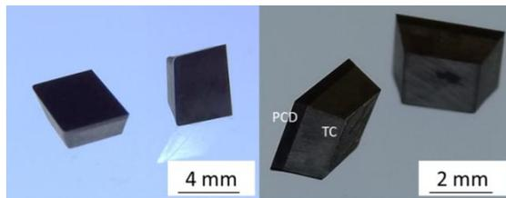
Figure 7: Examples for PCD samples of geometry 3 cut with the Laser MicroJet®.
