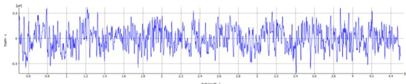
Figure 10: Example of roughness profile for measurement of the roughness on the top with Ra = 168 nm
