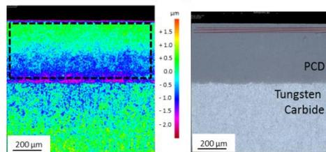
Figure 8: Example for a roughness measurement: Left: Image of measurement, Middle: Surface height of measurement with marked region for the measurement of the roughness on the PCD part.
