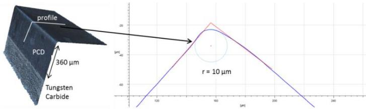
Figure 11: Right: Example for measurement to determine the radius of the tool cutting edge between the top surface of the PCD and the flank Left: Example for the measurement for the radius along a profile
