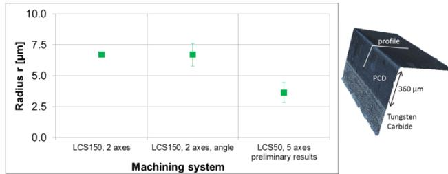
Figure 13: Cutting edge radius measurements PCD tools cut with the Laser MicroJet® technology depending on the cutting system and the number of axes employed
