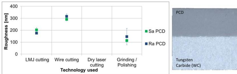
Figure 15: Comparison of the roughness on the kerf for PCD cutting tools processed using the conventional techniques of wire EDM cutting and mechanical grinding and with the Laser MicroJet<sup>®</sup> technology.
