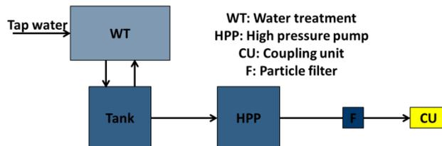
Figure 3: Sketch of water pump and water treatment.
