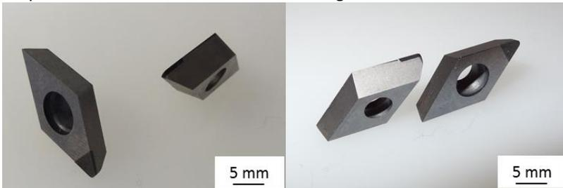
Figure 5: Picture of PCD tipped indexable inserts
