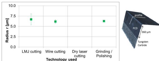
Figure 16: Comparison of the edge radius (sharpness) for PCD cutting tools processed with the conventional techniques wire cutting and grinding with the Laser MicroJet<sup>®</sup>.
