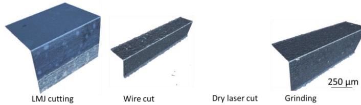
Figure 17: Comparison of the edge quality (sharpness) for PCD cutting tools processed with the conventional techniques wire cutting and grinding in comparison with the Laser MicroJet®.
