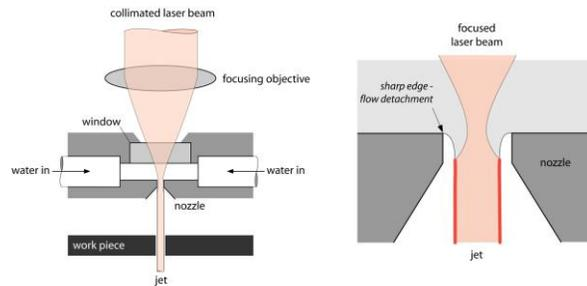
Figure 2: Sketch of the coupling of the laser into the water jet.
