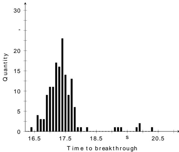
Fig. 2: Statistic distribution of 150 samples irradiated with a laser power of 3 kW and a beam diameter of 60 mm
