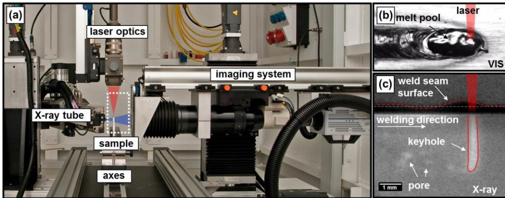
Fig. 3: (a) High-speed imaging X-ray system. (b) Single frame out of a high-speed observation of sample surface. (c) Single frame out of a high-speed X-ray observation of a weld [Abt, 2011].
