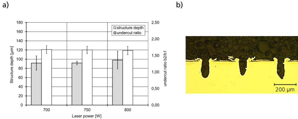
Fig. 9. a) analyzed geometric parameters for different laser powers for XSG; (b) cross section of microstructures for chosen parameter (laser power 800 W)
