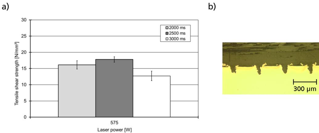
Fig. 11. (a) tensile shear testing results of XSG; (b) cross sections of joined specimen without any defects (575 W laser power and 2500 ms irradiation time)
