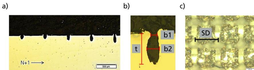
Fig. 7. (a) formation of the undercut groove by an increasing number of repetitions; (b) analysed geometric parameters of microstructures; (c) generated pattern on metal surface in form of crossed microstructures
