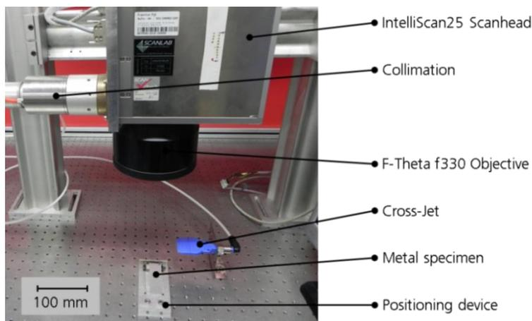
Fig. 4. system set-up for microstructuring process
