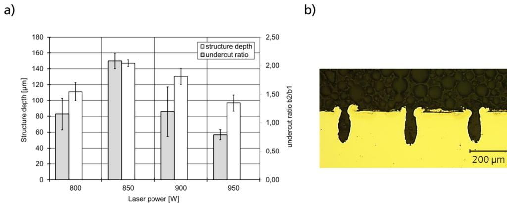
Fig. 8. (a) analyzed geometric parameters for different laser powers for P260; (b) cross section of microstructures for chosen parameter (laser power 850 W)
