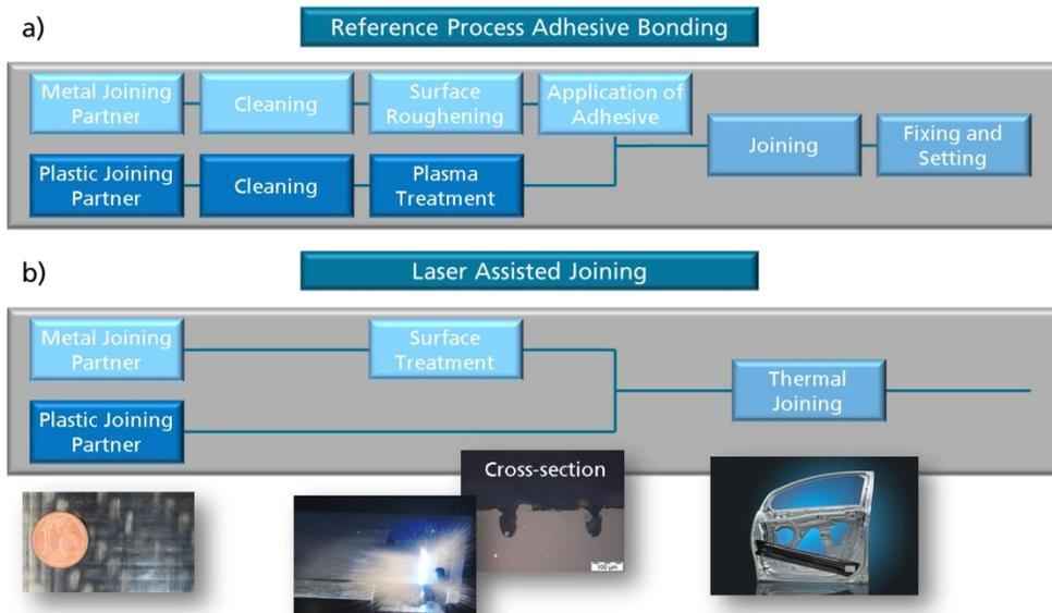
Fig. 1. comparison of two process chains for hybrid joints: (a) adhesive bonding; (b) laser assisted joining
