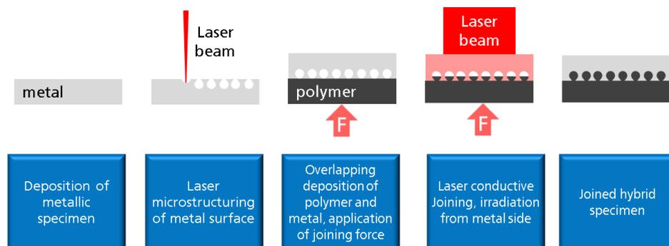
Fig. 2. laser based process steps: Microstructuring of metal surface and conductive joining from metal side
