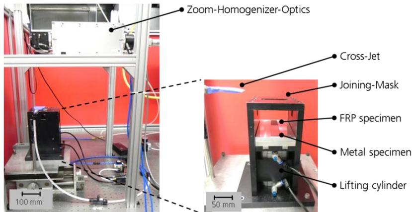
Fig. 5. system set-up for laser based conductive joining process
