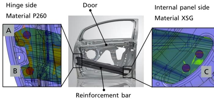
Fig. 3. PSA demonstration part with two joining areas A and B on hinge side (material P260) and one joining area C on internal panel side (material XSG)
