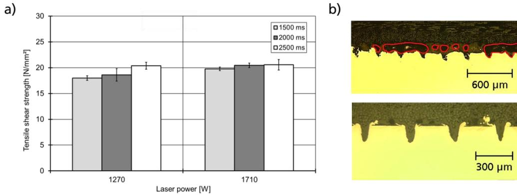
Fig. 10. (a) tensile shear testing results of P260; (b) cross sections of joined specimens with defects (1710 W laser power and 2500 ms irradiation time (top)) and without any defects (1710 W laser power and 2000 ms irradiation time (bottom))
