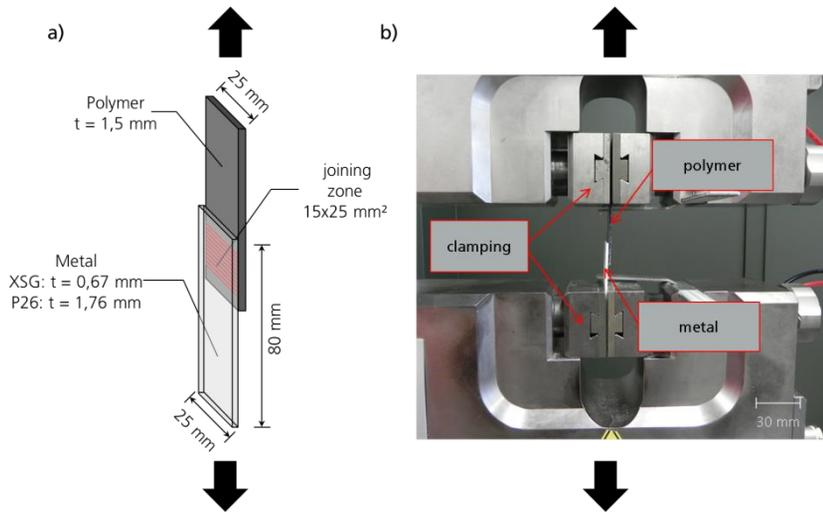
Fig. 6. (a) dimensions of tensile shear test specimens; (b) welded sample fixed for tensile shear test in testing machine
