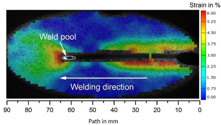
Fig. 5. Transverse strain distribution during welding at 3s, tested at a strain rate of 6%/s and at a strain 7%
