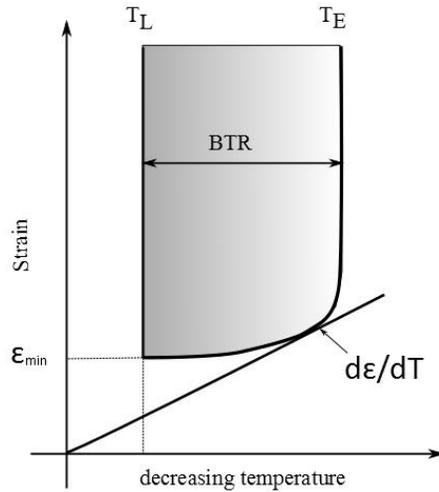
Fig. 1. The concept of brittleness temperature range (BTR) during solidification of metals in the strain-temperature regime Shankar et al., 2003
