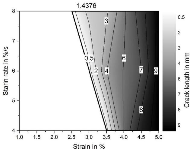
Fig. 4. Crack length as a function of the critical strain and strain rate for the steel grade 1.4376
