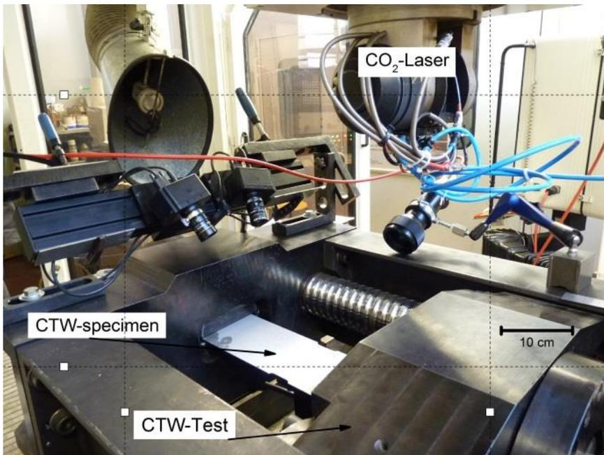
Fig. 2. CTW test facility used in conjunction with CO2 laser welding
