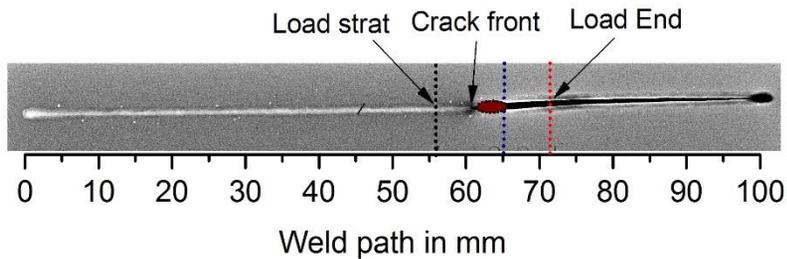
Fig. 6. Radiographic film showing centerline cracks in the CTW test specimen
