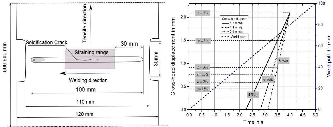
Fig. 3. The specimen geometry and a schematic illustration of the experiment
