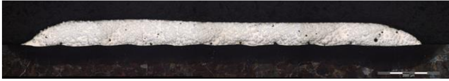
Fig. 3. Inter-run porosity in a coating with overlapped tracks
