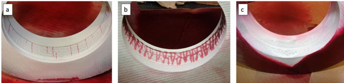
Fig. 6. Liquid penetrant tests on (a) preheated sample without buffer layer, (b) non-preheated sample with buffer layer and (c) preheated sample with buffer layer
