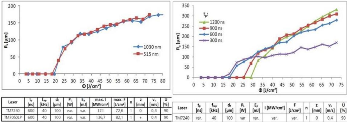
Figure 3: Left side: Structuring depth  $R_z$  as function of the fluence for the wavelengths 1030 nm (laser: TruMicro 7050 LP) and 515 nm (laser TruMicro 7240) as well as the applied laser parameters. Right side: Structuring depth  $R_z$  as function of the fluence for several pulse durations  $t_p$  as well as the applied laser parameters.  $F_{rep}$ : repetition rate,  $U$ : spot overlap,  $v_s$ : feed rate,  $t_p$ : pulse duration.
