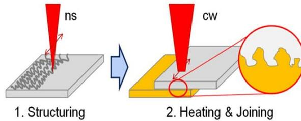
Figure 1: Principle of the joining process. A metal surface is structured with a nanosecond laser to form a big roughness and undercuts. The thermoplastic part is heated by a cw Diode laser. Melt of a thermoplastic part can flow into the structures to form a durable connection.
