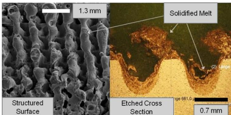
Figure 2: Microphotograph and etched cross section of a structured steel sheet
