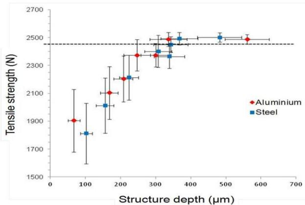
Figure 4: Tensile strength of aluminium / steel joints as function of surface structure depth.
