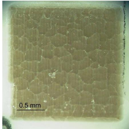
Fig 3. Optical image of a treatment made by the infrared source of the Nd:YVO<sub>4</sub> laser.
