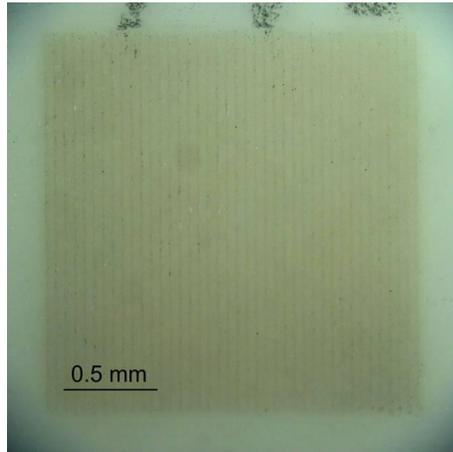
Fig 1. Optical image of a treatment by the ultraviolet source of the Nd:YVO<sub>4</sub> laser.
