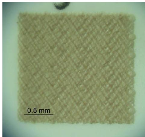
Fig 2. Optical image of a treatment made by the green source of the Nd:YVO<sub>4</sub> laser.
