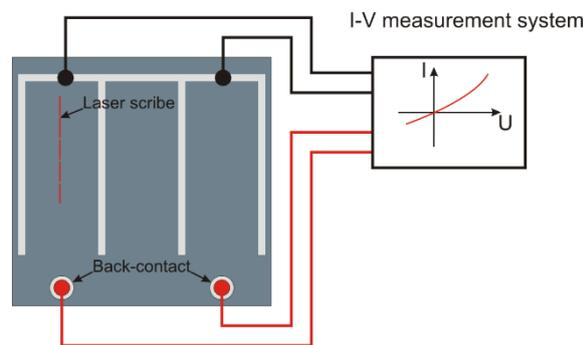
Fig. 2. Electrical measurement setup.
