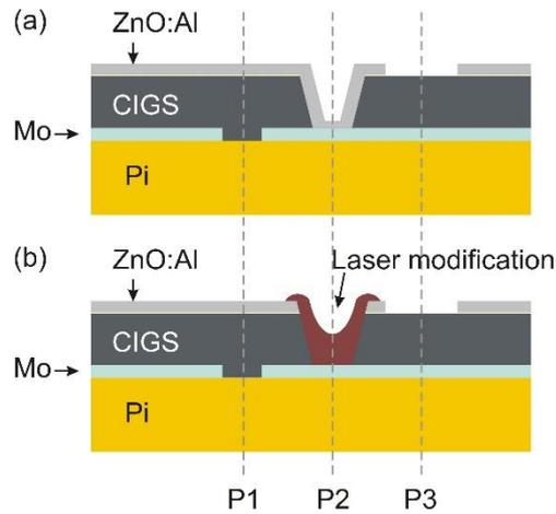
Fig. 1. (a) Conventional all laser scribed series interconnect in CIGS solar cell; (b) the series interconnect is formed via P2 micro-weld.
