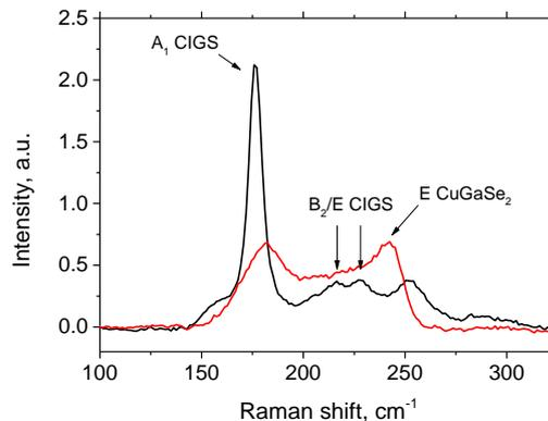
Fig. 4. Raman spectra of CIGS structure (black line) and laser modified P2 micro-weld area (red line).
