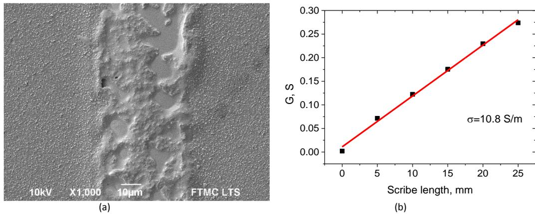
Fig. 3. (a) SEM image of P2 micro-weld in full CIGS structure, 0.1 J/cm<sup>2</sup>, 100 mm/s; (b) scribe specific conductivity measurement.
