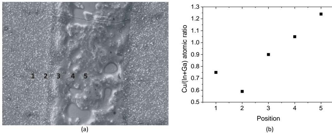
Fig. 5 (a) EDS spectra measurement positions near the P2 micro-weld; (b) Cu/(In+Ga) ratios in the measured positions.
