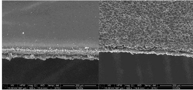
Fig. 1. SEM images of cut edges with parameter group 7 for cathode (left) and anode (right).
