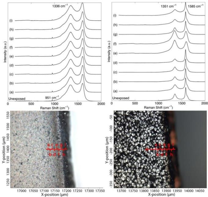
Fig. 2. Raman spectra and microscope images for cathode (left) and anode (right) with parameter group 7.
