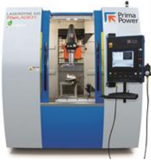
Fig.1. Experimental set-up; (a) 430 6-axis machining centre; (b) clamping fixture which produces constant pressure along the length of weld
