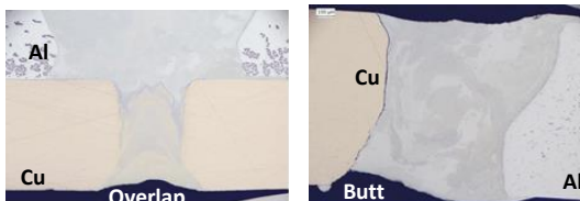
Fig.10. 1mm Al 3003+ 1mm pure Cu, 1.6kW power, \text{N}_2 shield, unetched micrograph
