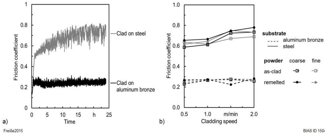
Fig. 2. Friction coefficient. a) Exemplary transient measurement data and b) average friction coefficient for the modified surfaces
