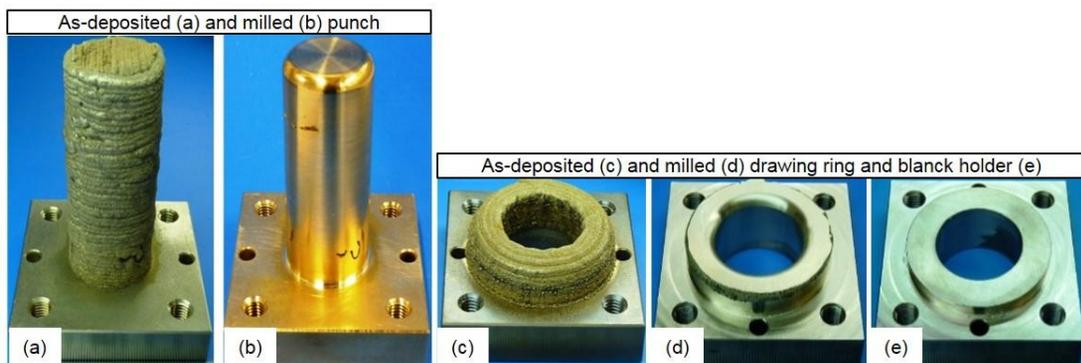
Fig. 3. Additively manufactured and milled deep drawing tool
