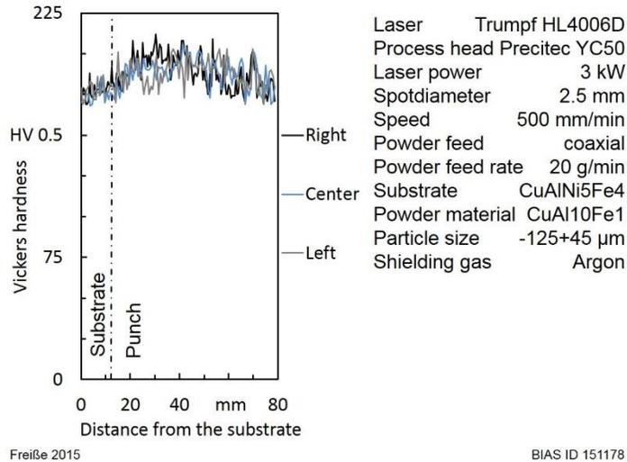
Fig. 4 Hardness distribution in the punch
