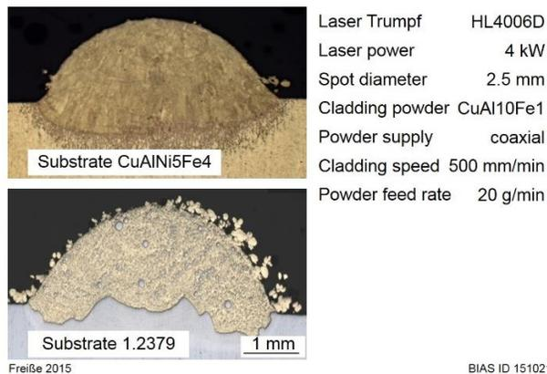
Fig. 1. Metallographic cross sections of laser cladded tracks on two different substrates
