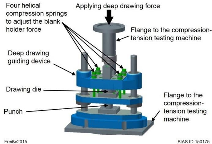
Fig. 5. Experimental set-up for the deep drawing test
