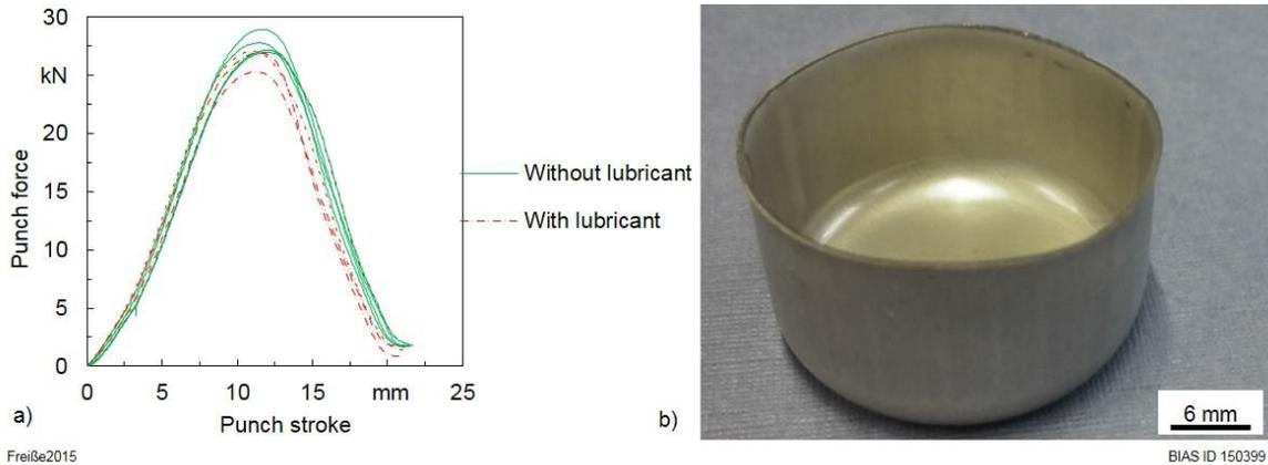
Fig. 6. Results of the deep drawing test with and without lubricant (a) and example of a dry formed cup (b)
