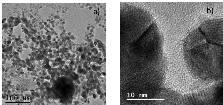
Fig. 2. Nanoparticles obtained by ablating Ag plate submerged in water with a pulsed laser: (a) TEM micrographs of Ag nanoparticles showing general appearance. (b) HRTEM of Ag nanoparticle showing clear fringes.
