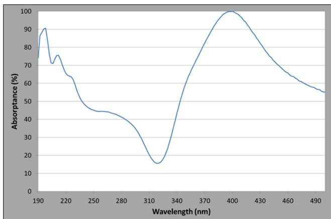
Fig. 3. UV-vis spectrum of colloidal nanoparticles obtained by laser ablation Ag plate submerged in water.
