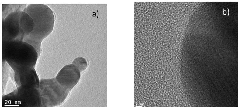
Fig. 1. Nanoparticles obtained by ablating Ag plate submerged in water with a CW laser: ( a ) TEM micrographs Ag nanoparticles appearance. ( b ) HRTEM of Ag nanoparticle showing clear fringes.
