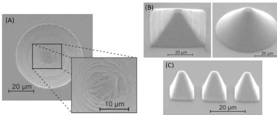
Figure 5: SEM images of a negative structure and elastomeric mold structures. (A) A low quality negative structure of a frustum, which generated cracks in the molding. The slope of the frustum was 46 degrees. (B) High quality molding structures of a pyramid and a frustum by changing the average laser power and scan velocity. (C) Generation of a pyramid array with one molding process.
