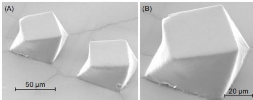
Figure 6: SEM images of a twisted truncated pyramid structure. These structures were elastomeric molded. The upper surface is twisted around about 45 degrees. The edge length of the base area is 50  $\mu\text{m}$ . The edge length of the upper base area was defined to three-quarter of lower base area.
