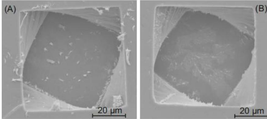
Figure 7: SEM images of twisted truncated pyramid structure in positive photoresist. The scan velocity was 0.1 mm/s. The average laser power was 5 mW. (A) shows considerable residuals of the elastomer from the molding process. (B) presents a superior molding quality in contrast to (A).
