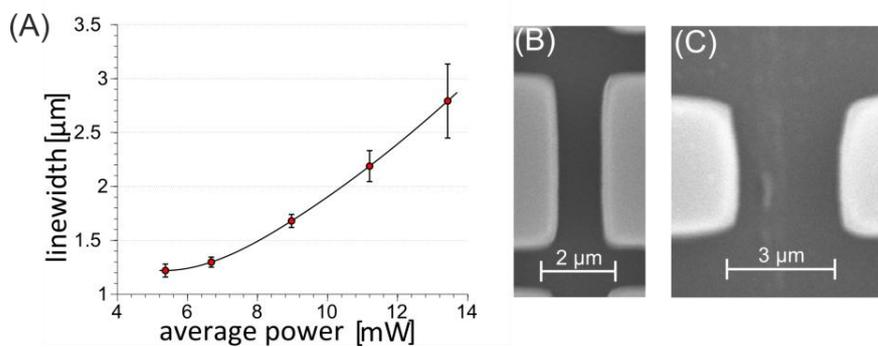
Figure 2: **Size distribution of the linewidth against average laser power.** (A) The scanning speed was  $0.95\ \text{mm/s}$  and the distance between the lines was  $5\ \mu\text{m}$ . The number of layers was 10 with an increment of  $500\ \text{nm}$  in z-direction. An SEM is used to measure the linewidth at the top of the structures. (B)-(C) presents the results of the effect of increasing laser power to the size of linewidth.
