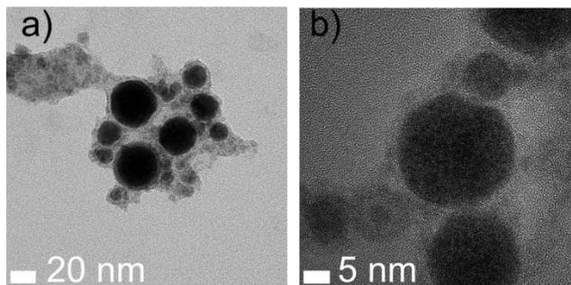
Figure 5: Nanoparticles generated in acetone at a) 800  $\mu\text{J}$  and b) 10  $\mu\text{J}$ .
