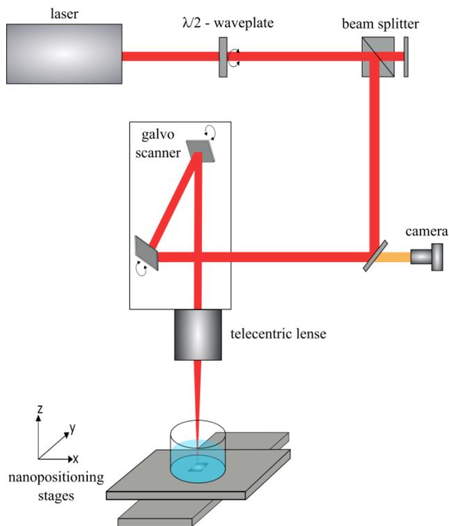
Figure 1: Scheme of the experimental setup for fs-PLAL in a batch chamber.
