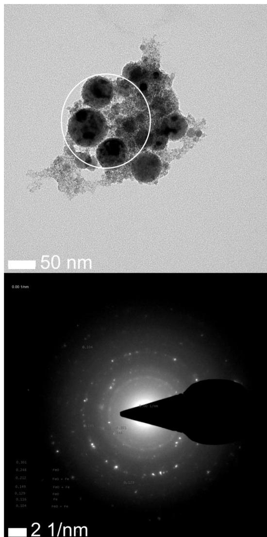
Figure 7: Nanoparticles generated in water (upper image) with the obtained SAED pattern (lower image).
