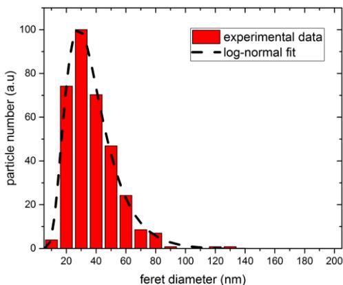
Figure 6: Feret diameter size distribution obtained from TEM pictures for a pulse energy of 800  $\mu\text{J}$  in water.
