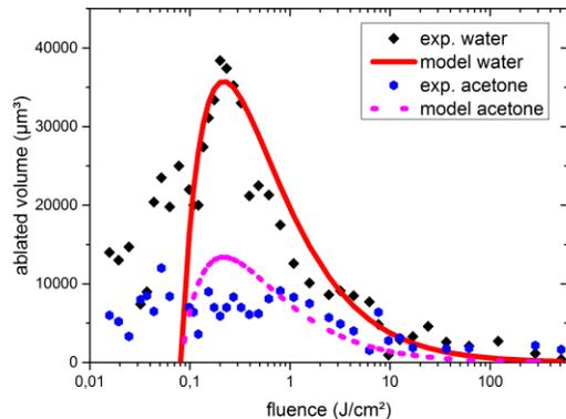
Figure 2: Ablated volume for 20 single shots for different fluences in water and acetone fitted with model curves.
