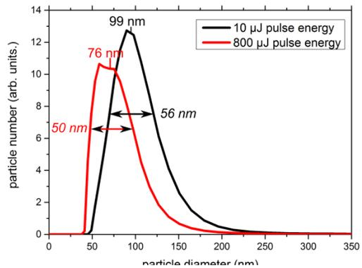
Figure 3: Size distribution of hydrodynamic nanoparticle diameter generated at different pulse energies for optimal ablation conditions at 800  $\mu$ J and 10  $\mu$ J.
