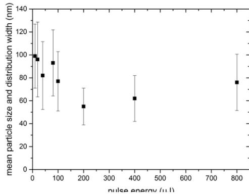
Figure 4: Mean particle size and distribution width of a lognormal fit to the obtained hydrodynamic size distributions generated at different pulse energies.
