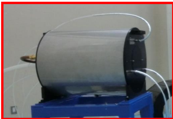
Fig. 3 Power meter developed for 100 kW.
