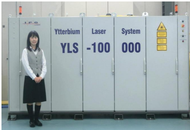
Fig. 1 100 kW fiber laser apparatus used.
