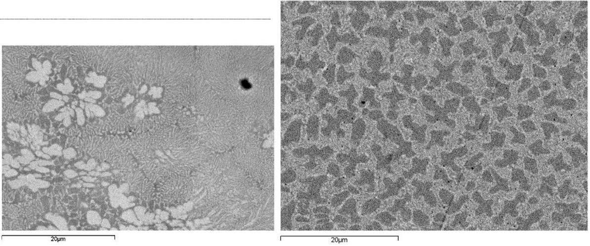
Fig.3. Detail of microstructure after metal deposition as seen by SEM (retro-dispersed electrons): (a) T800 (b) T 900
