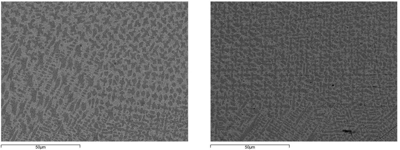
Fig.4. Microstructure of deposited T800+Ni20Cr mix as seen by SEM (retro-dispersed electrons).
