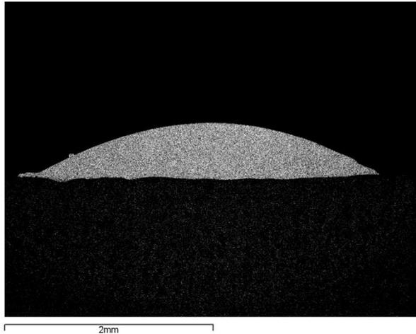
Fig. 1. (a) Cross sectional view of bead profile obtained with T900 (3.6 g/l) powder at P=1250 W and v= 3 mm/s .
