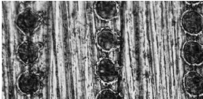
Figure 1. Cu, single pulse, 1ns laser, 10 \mu J pulse energy, 10 \mu m diameter
