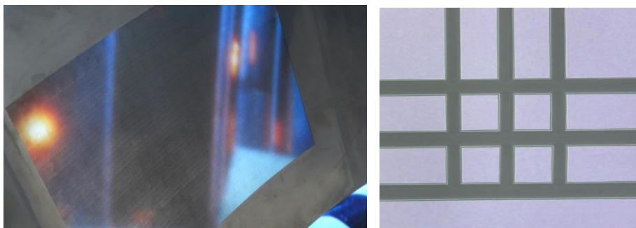
Fig. 5: Multibeam drilling of filter foils (left), Multibeam thin film ablation of ITO-layers (right)
