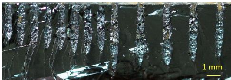
Fig. 2. Side view of the silicon slab of 7.5 mm thickness with holes drilled with single burst of energy 2.6 J to 4.46 J (from left) and with six bursts with increasing energy from 4.46 J to 3.39 J in experiment with drilling resonator.
