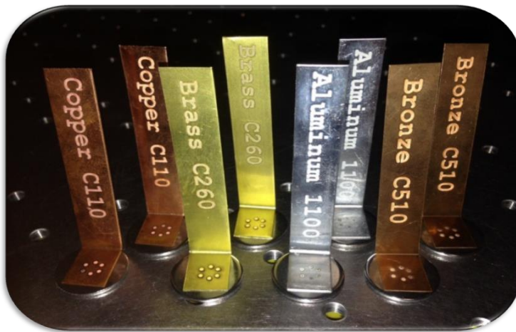
Fig. 1. Examples of various metals welded to stainless steel.
