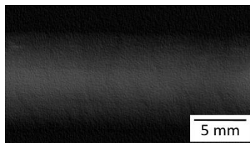
Fig. 4. Radiograph (top view) of a pyramid structure without macroscopic defects laser metal deposited at room temperature.
