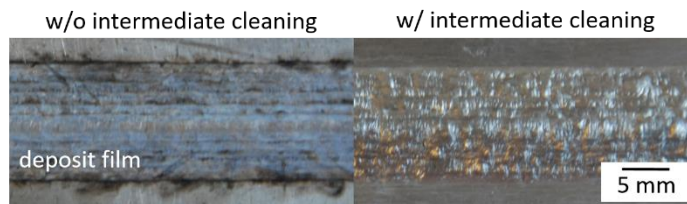
Fig. 2. Surface appearance (top view) of a laser metal deposited pyramid structure at room temperature without and with intermediate cleaning after each deposition of a bead.
