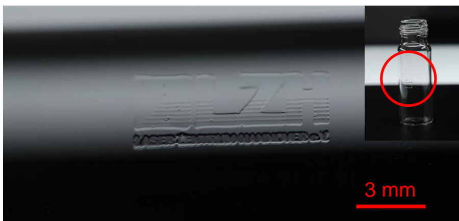
Fig. 10. LZH logo ( 3.00 \times 8.07 \text{ mm}^2 ) printed on a freeform cylindrical surface with an outer diameter of 14.8 mm
