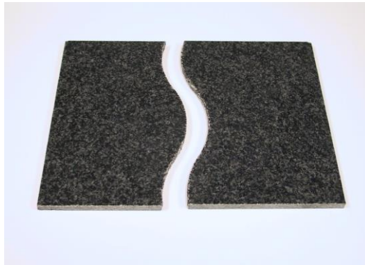
Fig. 5. Viability of laser cutting to produce complex shapes in Zimbabwe black granite.
