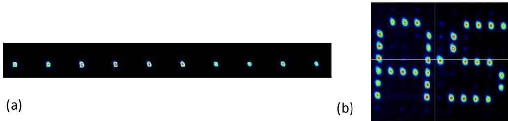
Fig. 2: example of beam intensity distribution after multi spot beam shaping with a YUJA laser from Amplitude Systèmes ( $100 \mu\text{m}$  at 100 kHz) and the Qjova head.
