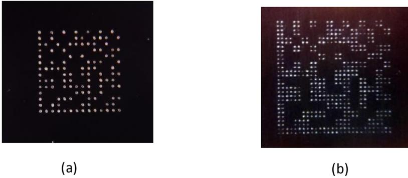
Fig. 4: example of multi spot marking with one laser pulse of 5 mJ. (a) silicium, (b) stainless steel for spot density x4
