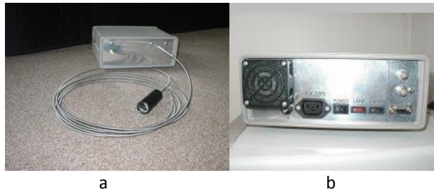
Fig. 3. Control unit with optical head-(a). Rear panel of the control unit – (b).
