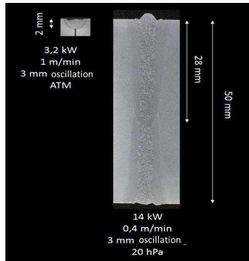
Fig. 11. Micrograph sealing weld (left) and joining weld (right), MoVak, 20 hPa
