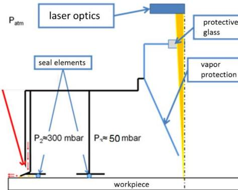
Fig. 8. Schematic setup of the mobile vacuum chamber
