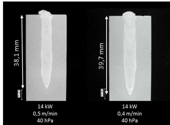
Figure 11. Micrograph butt weld aluminium, MoVac, 15 hPa
