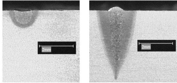
Fig. 3. Change in welding seam geometry atmospheric pressure (left), 10 hPa (right), 600 W
