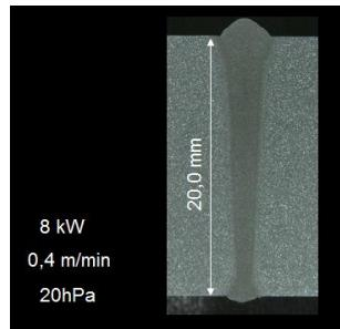
Fig. 10. Micrograph through weld, MoVac, 20 hPa
