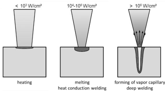
Fig. 1. Transition from heat conduction to deep welding
