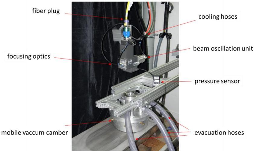
Fig. 7. Experimental setup of the mobile vacuum system for laser beam welding
