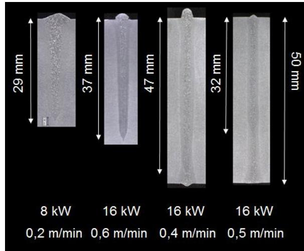
Fig. 9. Micrograph through bead-on-plate weld (left) connection weld (right), MoVac, 50 hPa
