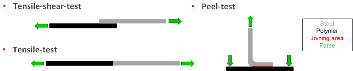
Fig. 8. Samples geometry for different types of stress
