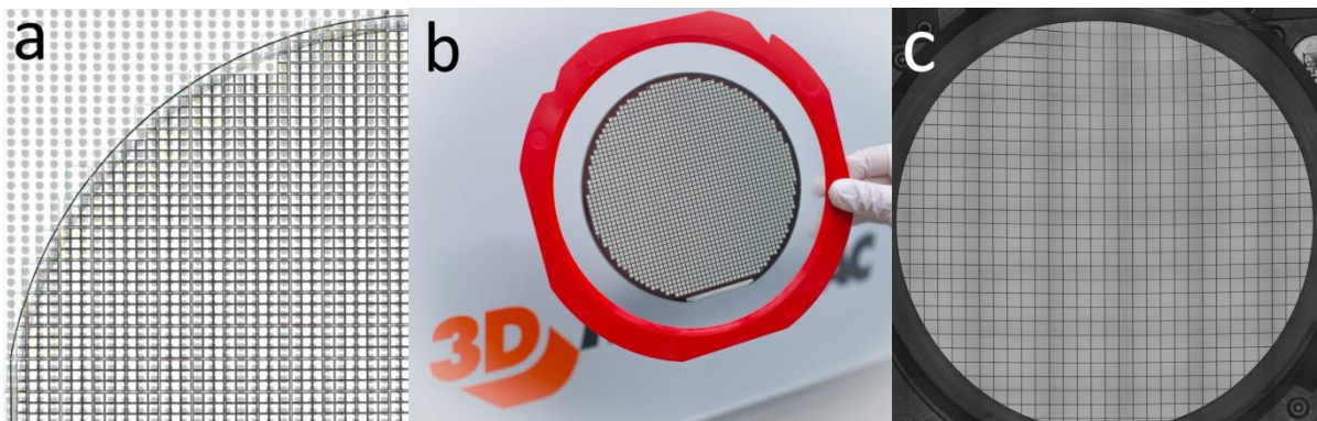
Fig. 3. (a) Diced quarter of 4-inch SiC wafer; (b) 4-inch SiC wafer; (c) mapping of diced 6-inch SiC wafer
