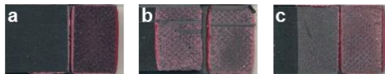
Fig. 2. Representative fracture patterns: (a) adhesion failure (AF); (b) cohesion failure (CF); (c) substrate close cohesion failure (SCF)
