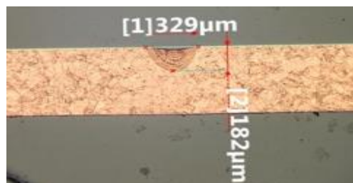
Fig. 9b. Cross section results for 500 \mu\text{m} Copper @ 275 Watts, 0.3 m/min – conduction mode
