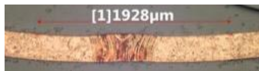
Fig. 9a. Cross section results for 500 \mu\text{m} Copper @ 275 Watts, 0.06 m/min – keyhole mode Regime
