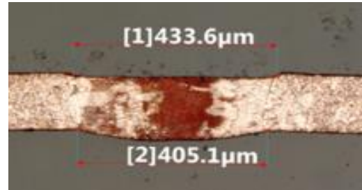
Fig. 5b. Cross section results for 125 μm Copper @ 275 Watts, 4.8 m/min
